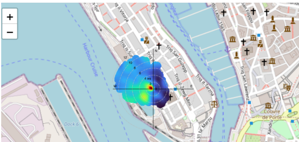
Geolocated polar plot showing the relationship of incidence of high BC concentration in Isla with wind speed and wind direction
