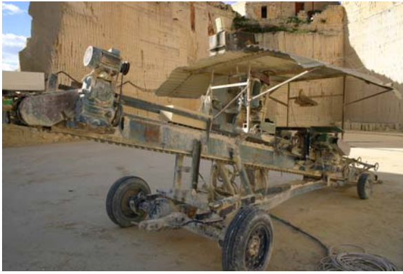
Figure 3. Typical dressing machine as used in softstone quarries.
