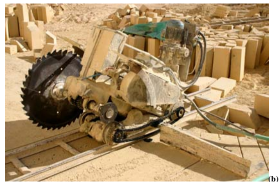
Figure 2. Typical cutting machines as used in softstone quarrying: (a) machine used to make horizontal cuts through bedrock and (b) machine used for vertical cuts.
