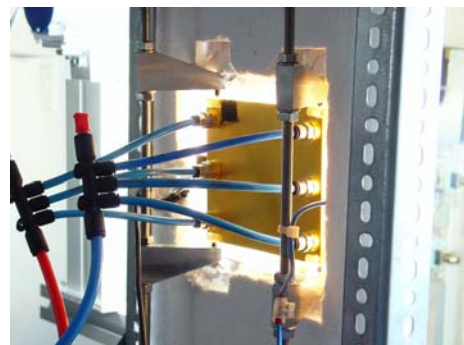
Figure 5. Water-cooling system of the CCM.
