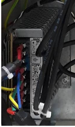
Figure 6.10: Mean Well RQ-50C - Supplies the PCBs for the Buck Converter
