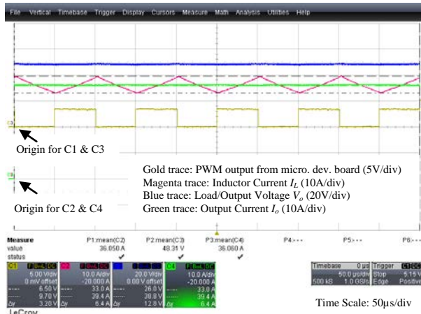
Figure B.15: Buck Converter – Open Prototype – Steady State R_{load} = 1.3\Omega, I_o = 36A
