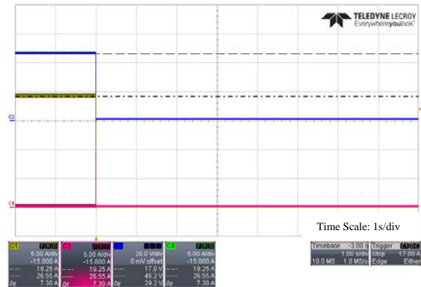
Figure 7.53: Paralleled Buck Converters – V-I Droop – Buck 1 Switching Off – Resistive Load R_{load} = 2.4\Omega
