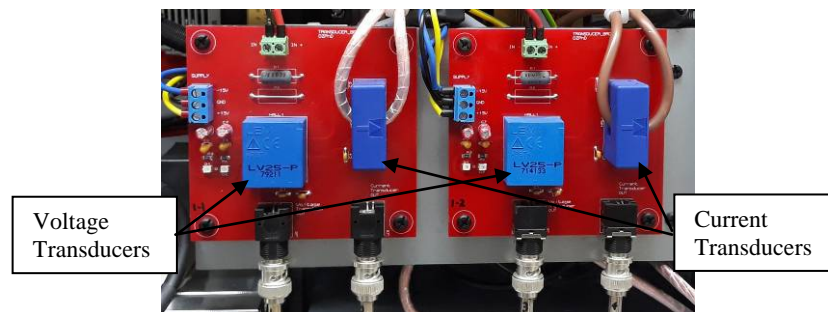
Figure 6.12: Transducer PCBs in the Buck Converter
