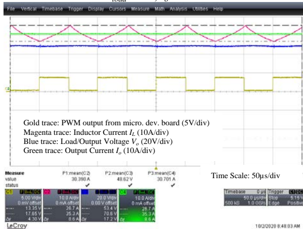
Figure B.10: Buck Converter – Open Prototype – Steady State R_{load} = 1.6\Omega, I_o = 30A
