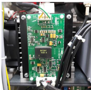
Figure 6.28: IGBT Driver PCB for the Buck Converter
