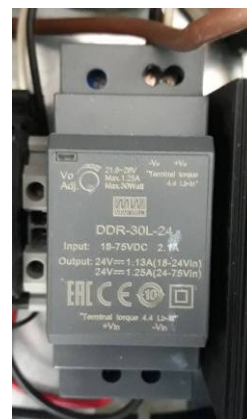
Figure 6.40: Mean Well DDR-30L-24 - Supplies the Contactor Coils and the Heatsink Fan for the Bidirectional Converter
