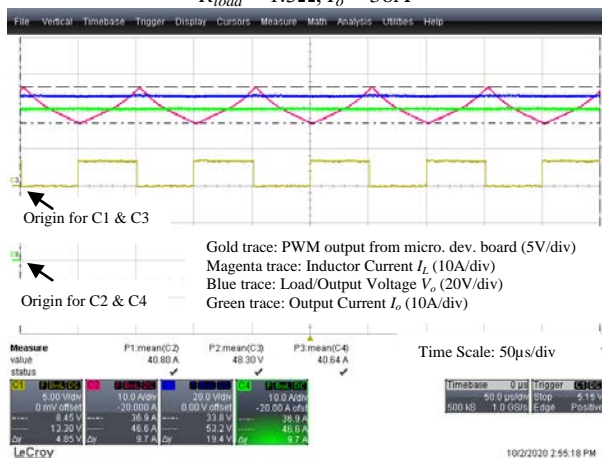
Figure B.17: Buck Converter – Open Prototype – Steady State R_{load} = 1.2\Omega, I_o = 40A
