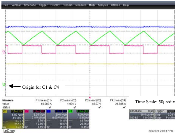
Figure B.59: Bidirectional Converter – Buck Mode – Steady State – Battery Supply – Load Supplying R_{load} = 4.8\Omega , I_o = 10A
