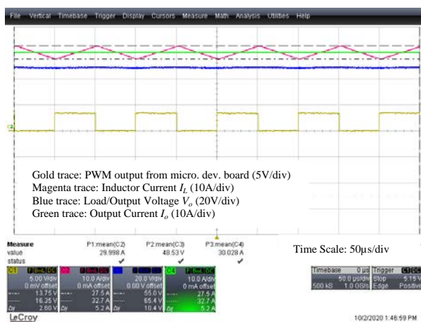
Figure B.13: Buck Converter – Open Prototype – Steady State R_{load} = 1.6\Omega , I_o = 30A
