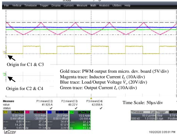
Figure B.19: Buck Converter – Open Prototype – Steady State R_{load} = 1.14\Omega, I_o = 42A
