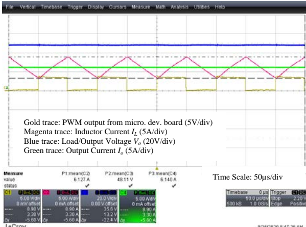
Figure B.2: Buck Converter – Open Prototype – Steady State R_{load} = 8\Omega, I_o = 6A
