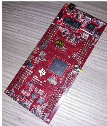
Figure 6.64: TI LaunchPad LAUNCHXL-F28379D Development Board with TMS320F28379D microcontroller
