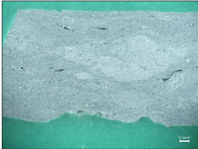
Figure 4.16 – 63_700_30_Red embedded briquette cross-section at a magnification of x10.
