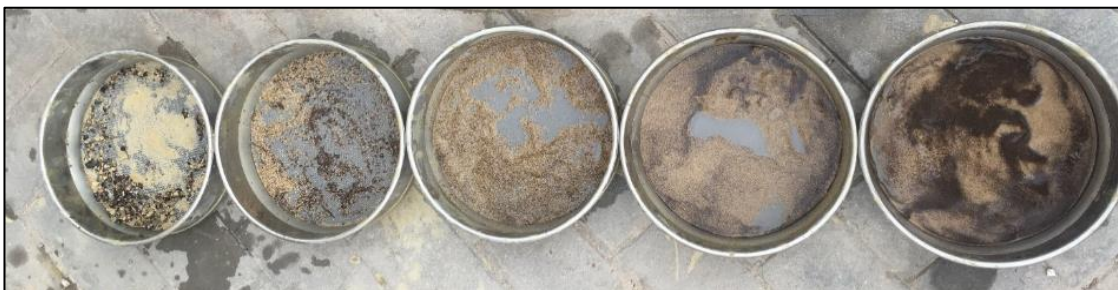
Figure 3.3 – Clay, soil, and rock particles in the different sieves. From left to right – 1 mm sieve, 500 \mu\text{m} sieve, 250 \mu\text{m} sieve, 125 \mu\text{m} sieve, and 63 \mu\text{m} sieve.
