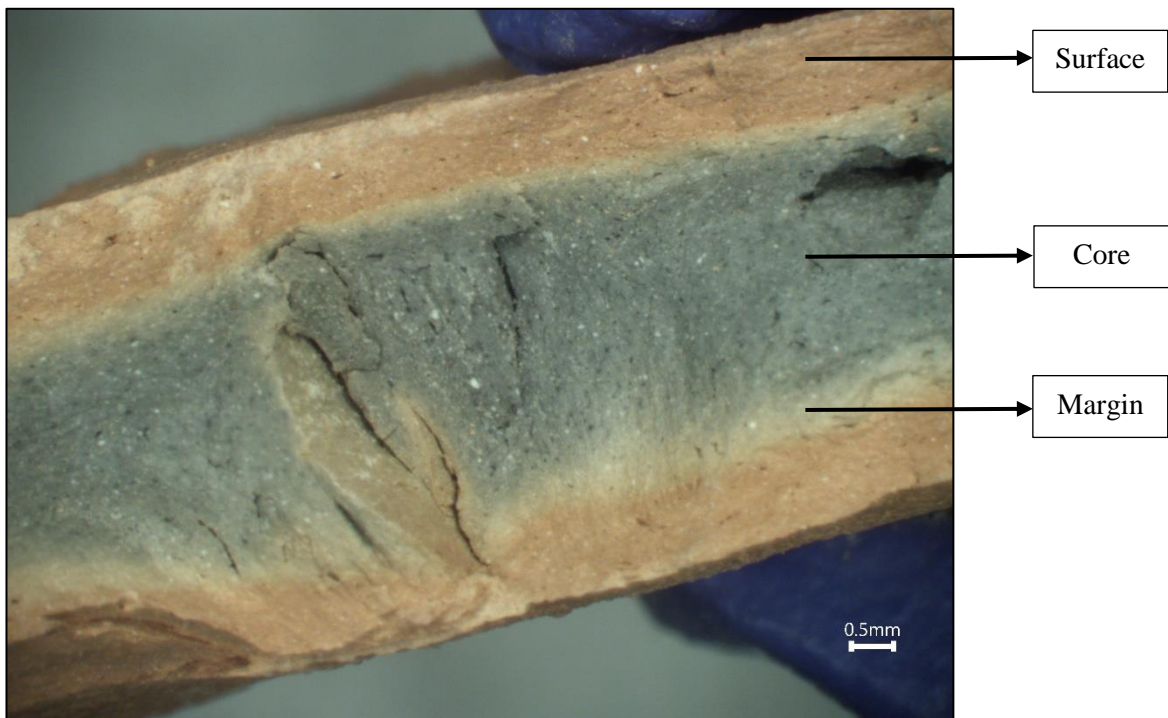
Figure 3.6 – A cross-section of one of the fired briquettes showing the different colours of the surface, core, and margin.
