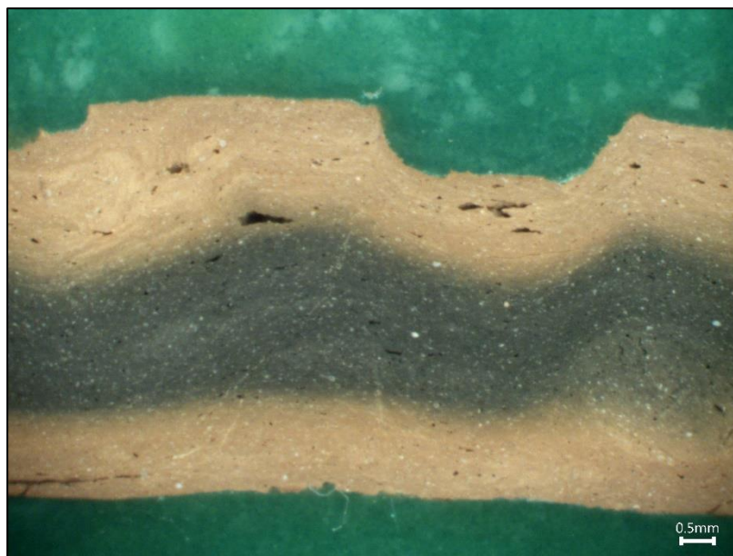
Figure 4.8 – 63_500_120_Oxi embedded briquette cross-section at a magnification of x10.
