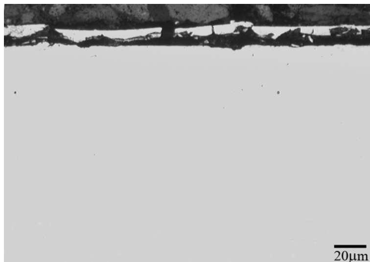
Figure 4-3.7.2 Cross-Section micrograph (polished) of ASTM F1586 sample carbo-nitrided at 430°C (NN430) after crevice corrosion immersion test
