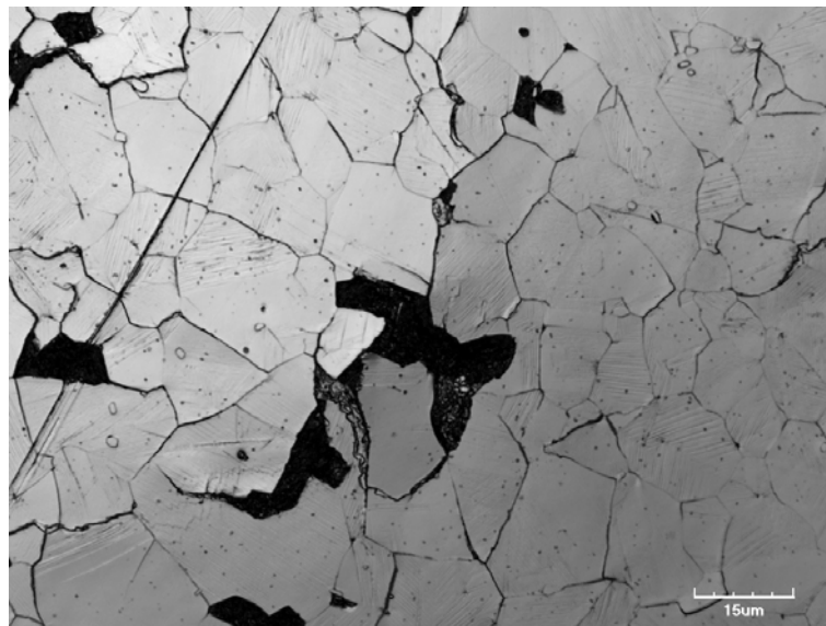
Figure 4-3.7.1 (d) Zoomed in laser confocal microscope detail (2-D intensity mode) from Figure 4-3.7.1 (a) showing grain pullout.
