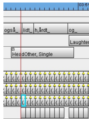
Figure 4: Area in Annotation window showing from top to bottom the manual annotation for the HeadOther movement in the previous figure, three tracks of frame-by-frame annotations for velocity, acceleration and jerk, and the annotation predicted by the SVM model. It can be seen that the Laughter annotation also coincides with a predicted head movement.
