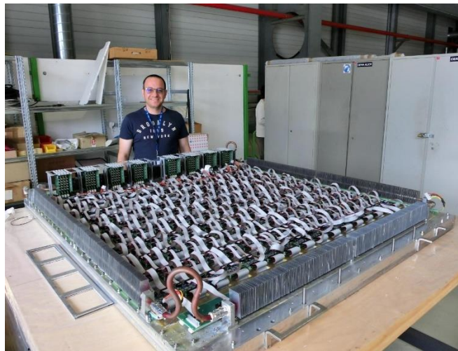
Figure 3: Illustration of one CPV module consisting of 7680 analogue channels, having an area of 200 x 230 cm 2 .
