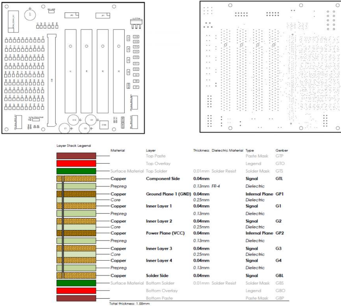
Figure 65: 8-layer PCB Board Stacking for Segment card.
