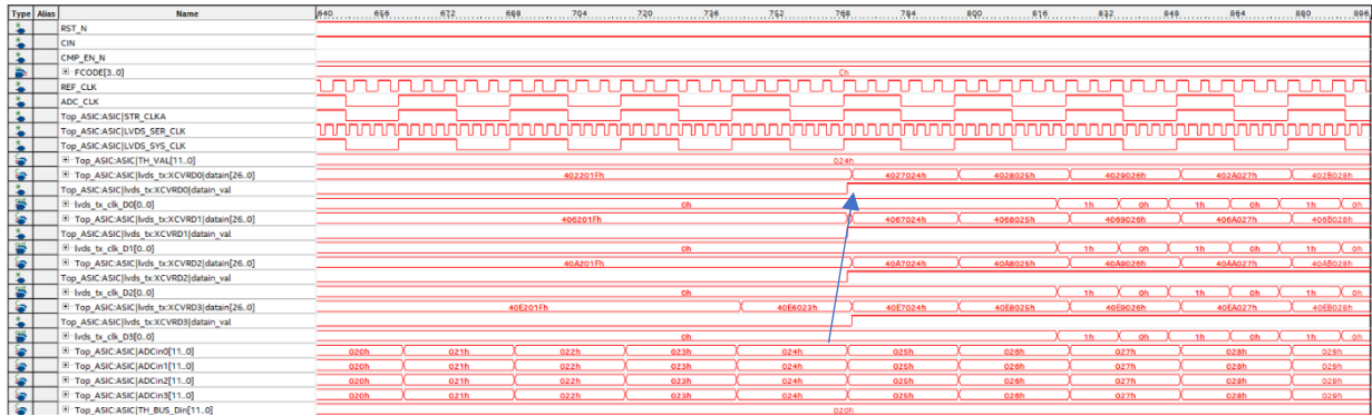
Figure 107: Digital codewords greater than a set threshold 0x24 on port TH_VAL<11:0> are transmitted, on setting CMP_EN. In this test bench, LVDS_SYS_CLK is set to 10MHz, while LVDS_SER_CLK is 90 MHz. The least significant bit (LSB) is transmitted first. The function of the input CMP_EN_N is for data suppression. Only values greater than a specified threshold at TH_VAL < 11:0 >, are transmitted over the LVDS ser connections, suppressing unwanted analogue codewords or noisy channels. The internal DSPR FIFOs are only activated if the ADCin<x><11:0> data is greater than 0x24, which is signalled by the datain_val control bit, where x represents a value from 0 to 3.
