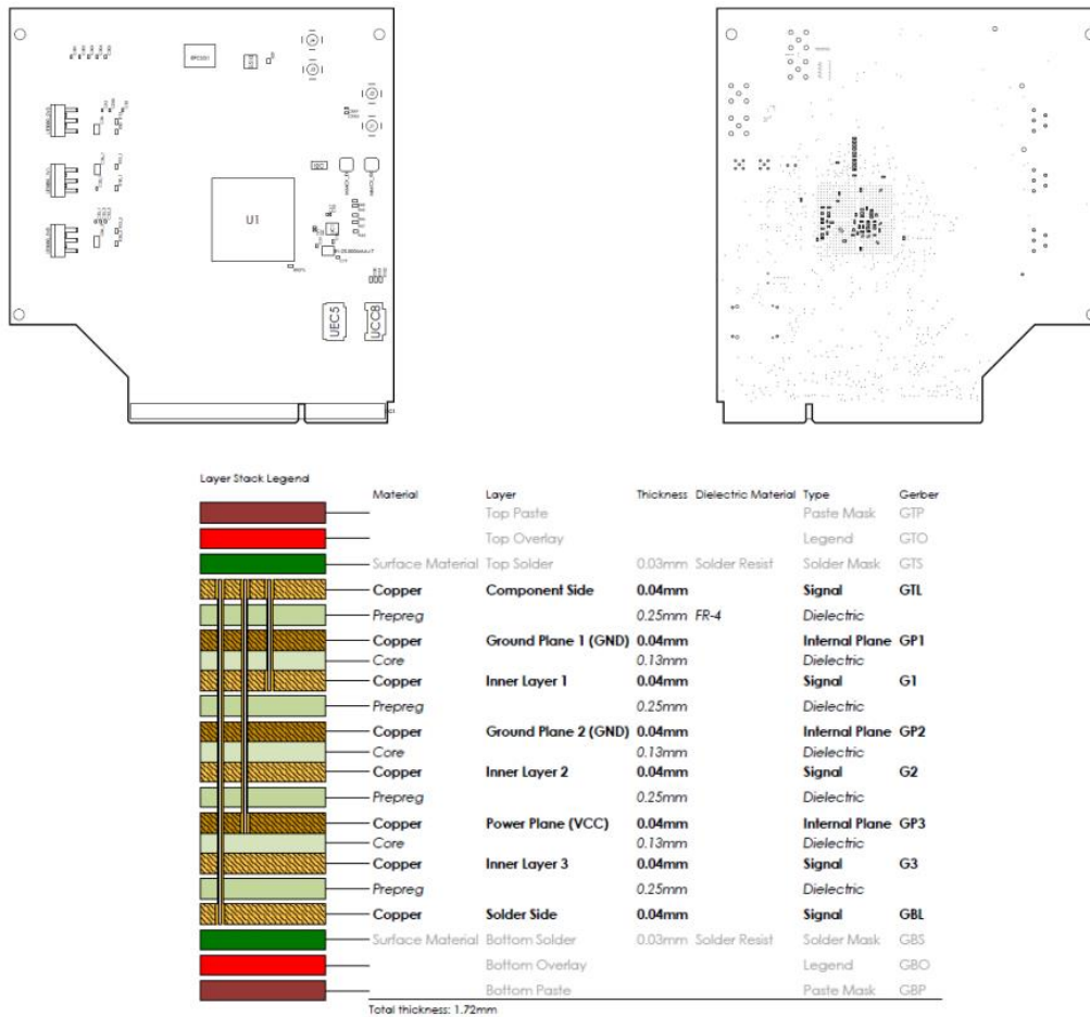
Figure 54: Column Controller PCB Board Layer Stacking.
