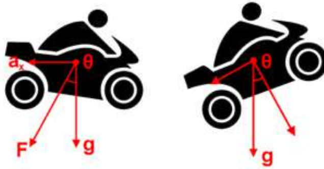
Figure 6.1: Motion cueing to physically emulate the motorcycle ride
