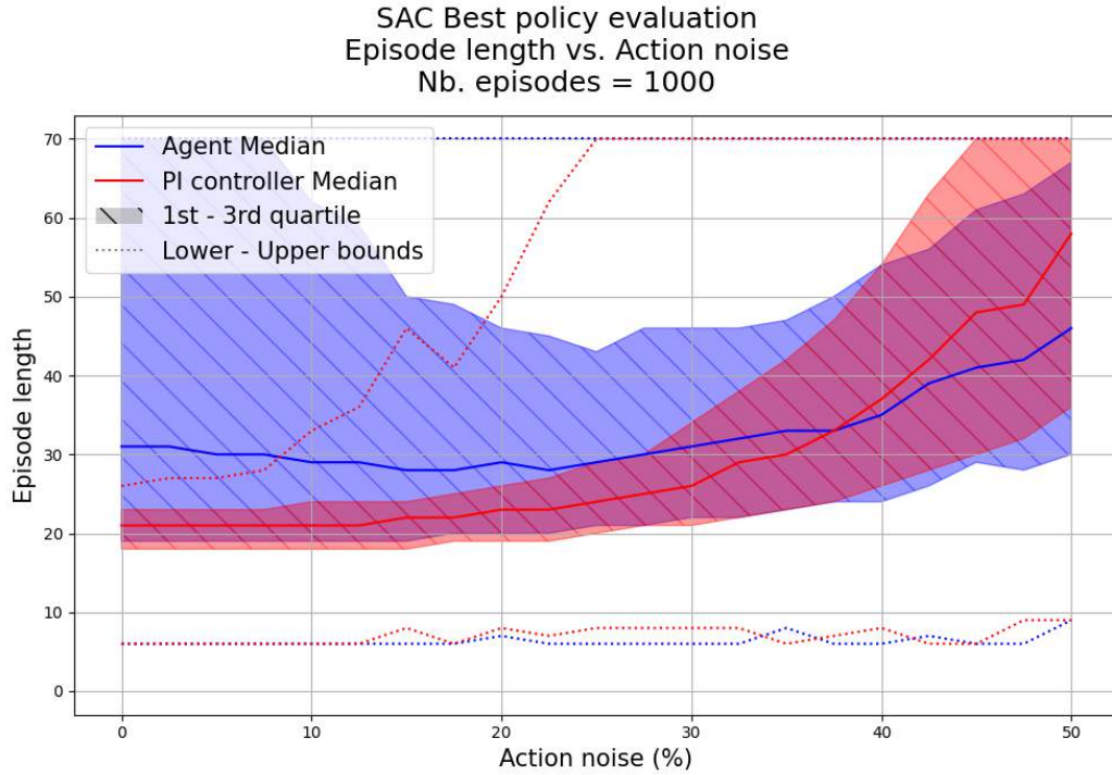
Figure 4.34: Effect of action noise on the episode length due to varying action noise on the best SAC agent and the PI controller.
