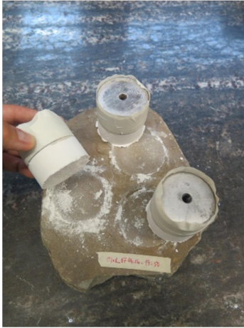
Figure 3. Assessment of the adhesion of the grout to the tuff stone support. © Gvantsa Potskhishvili, 2015.
