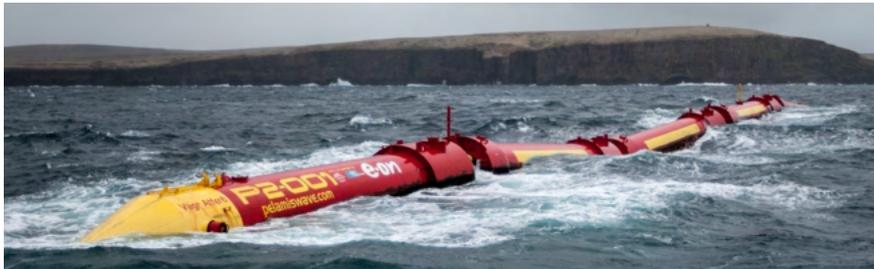
FIGURE 2.14: *Pelamis Wave Power WEC [Image by EMEC]*
