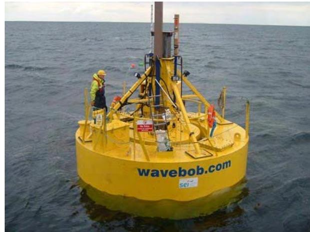
FIGURE 2.6: 1:4 Scale Wavebob model [49]
