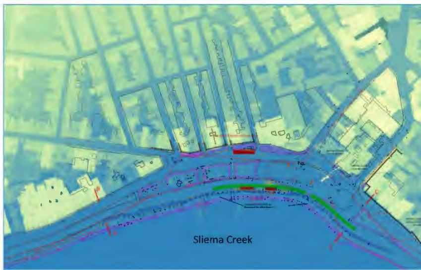
Figure 3: Superimposition of the road layout onto the DEM generated from LiDAR
