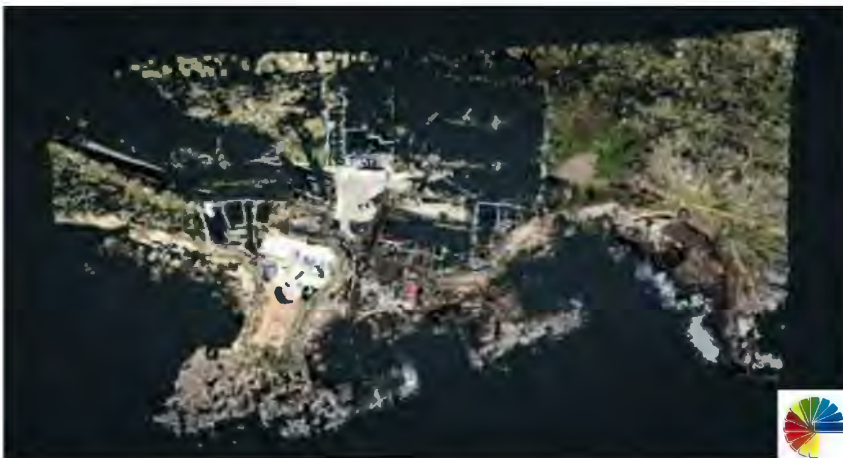
Figure 4: TLS LiDAR terrestrial (lacks building roofs)
