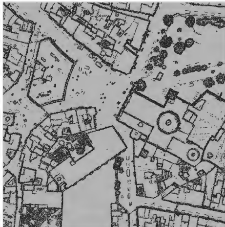
Figure 1: Height raster shows the identified wall pixels
