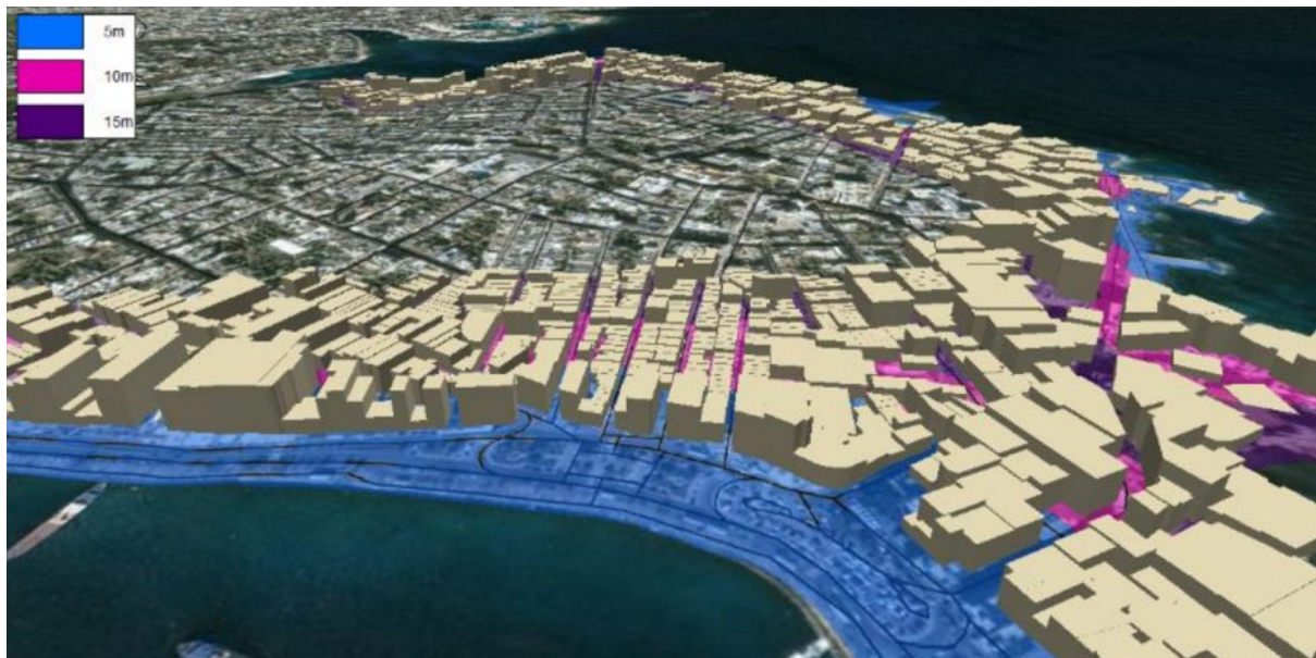
Figure 2.19 – 3D visualization of The Strand Sliema displaying the three levels of inundation (Source: Attard (2017)).
