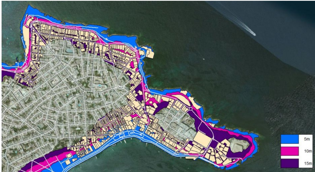
Figure 2.18 - 2D visualization of Sliema area displaying the three levels of inundation (Source: Attard (2017)).
