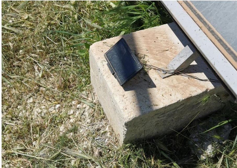
Figure 4.9: Solar shading occurrence due to a metal structure surrounding the installation area.
