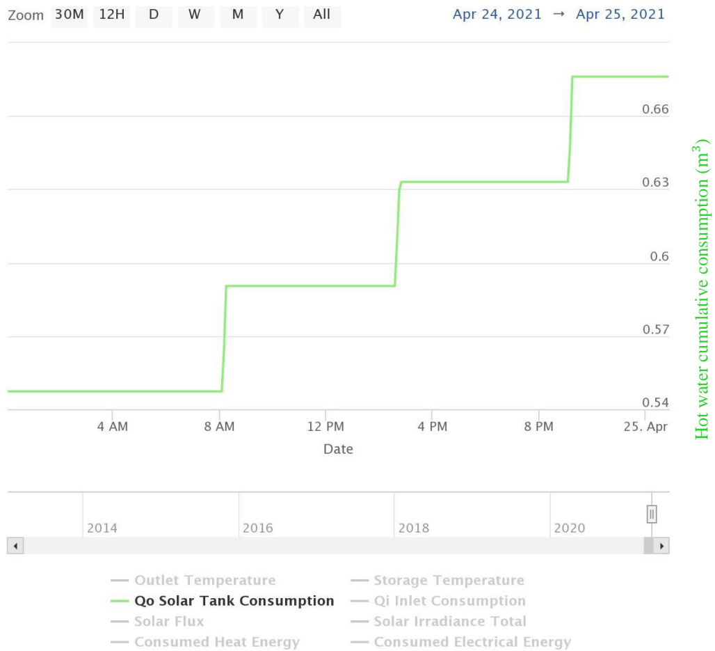
Figure 4.10: Qo Solar Tank Consumption trend showing instances of hot water consumptions for the 24th of April 2021.
