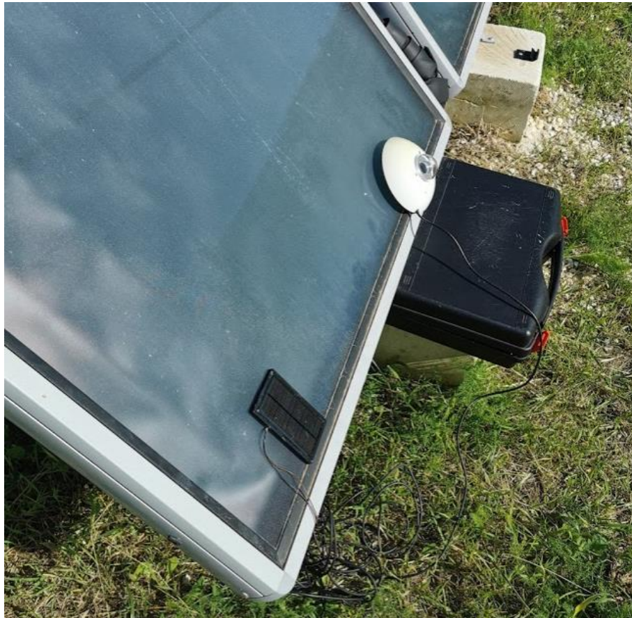
Figure 3.9: Solar Irradiance calibration setup
