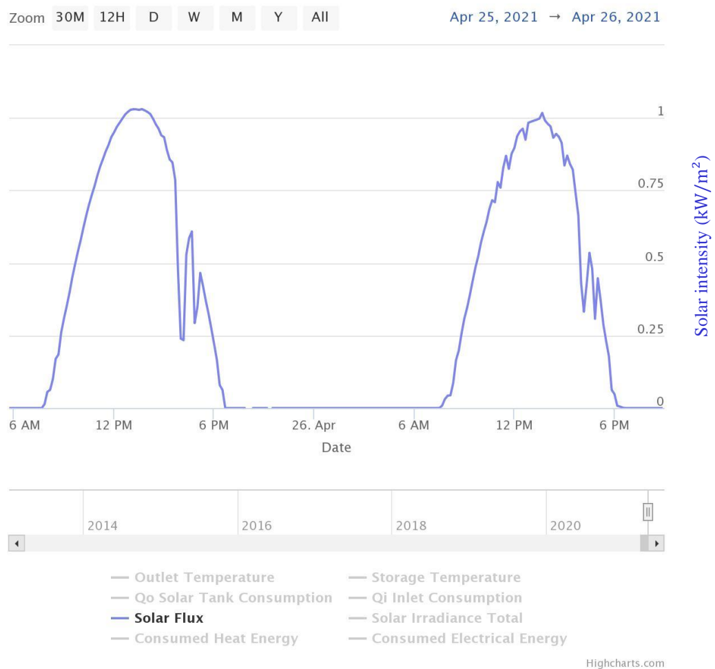
Figure 4.8: Solar shading effect on solar irradiance readings. Charts showing solar irradiance (in kWh/m 2 ) for the 25 th and 26 th of April 2021.
