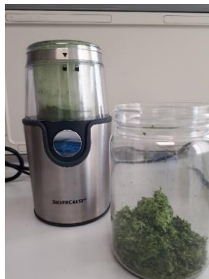
Fig. 2.18 Silvercrest coffee grinder was used to grind Alaria esculenta and Lemna minor into fine powders. Plastic tub on the right contains unground Lemna minor .
