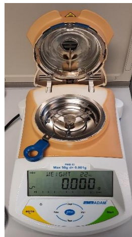
Fig. 2.8 The moisture analyzer, PMB 53, Adam, United Kingdom.
