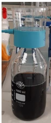
Fig. 2.36 The Bradford's reagent after being filtered through a 0.22 µm vacuum filter unit.
