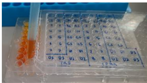
Fig. 2.47 Standards/samples being placed in a 96-well plate.
