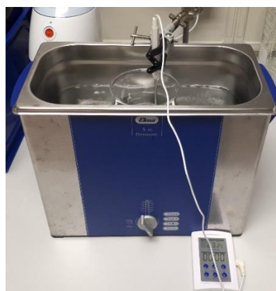
Fig. 2.14 The set-up of the bath sonicator.
