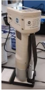
Fig. 2.1 Calibrating the colorimeter against a white tile.
