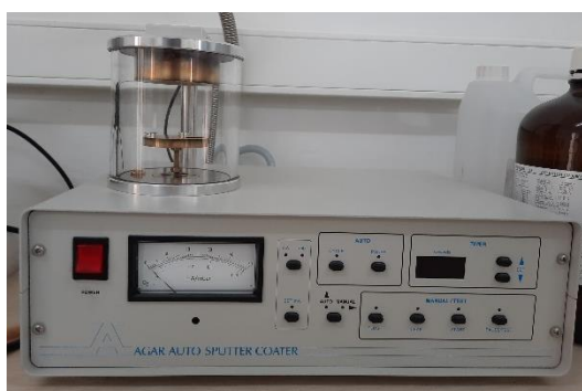
Fig. 2.53 The automatic sputter coater with two stubs holding samples fitted in the holders.
