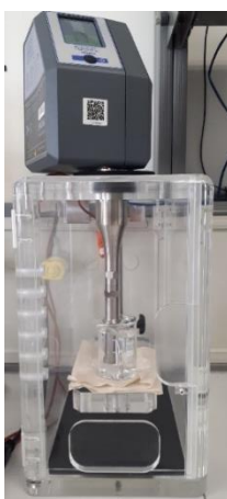
Fig. 2.17 The set-up of the UP400St probe sonicator.
