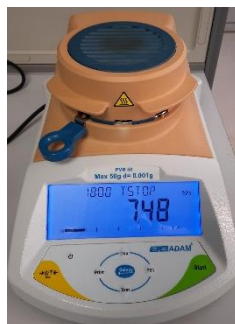
Fig. 2.13 The end result (% moisture) was seen on the display screen.
