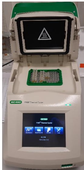
Fig. 2.46 Standards and samples inside the thermal cycler (T100, BioRad, Malta).
