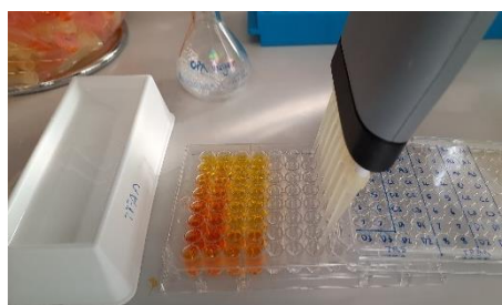
Fig. 2.42 OPA reagent was added to the samples by using a multichannel micropipette.
