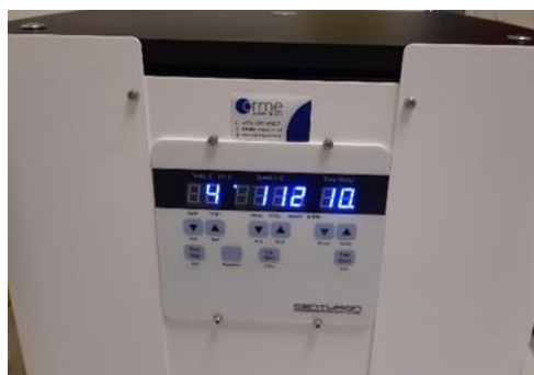
Fig. 2.52 The centrifuge set for 10 min at 1,120 RCF (g-force) and 4°C.
