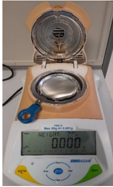
Fig. 2.10 The aluminium pan was weighed and tared.
