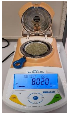
Fig. 2.11 The aluminium pan was filled with 8 g of sample.
