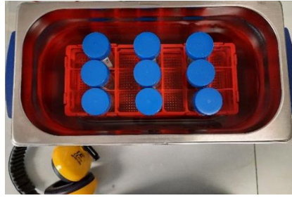
Fig. 2.24 The set-up for the treatment with the bath sonicator. The 50 mL centrifuge tubes were held upright and in place with the aid of a rack placed inside the tank. On the bottom left there is the ear protection used during all ultrasound treatments as a precaution.
