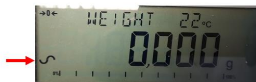
Fig. 2.9 The stable sign ~ is seen once the machine reaches a stable internal temperature.
