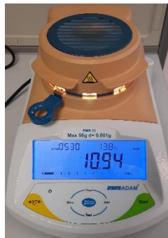
Fig. 2.12 The lid was lowered and the once the process started, light was emitted from the red-hot filament.
