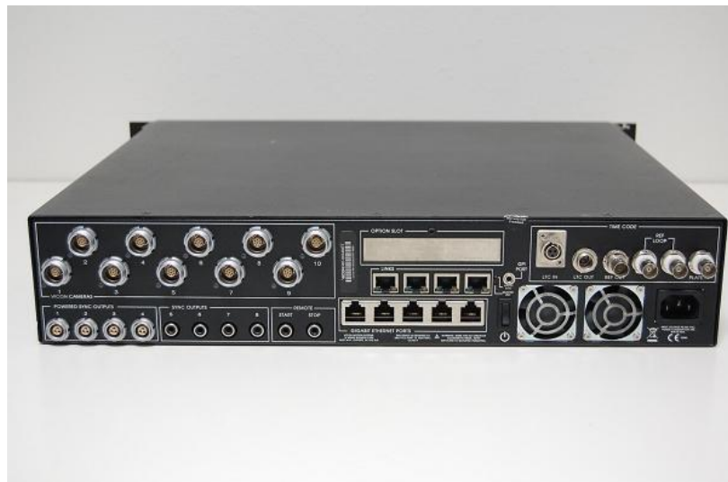
Figure 3.28: Vicron Giganet rear view, showing all camera and network connections
