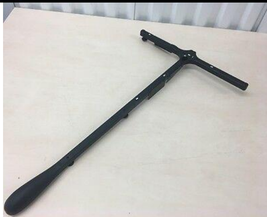
Figure 3.35 a and b: Calibration Screen and Calibration Wand
