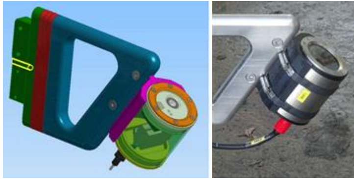
Figure 13: Camera system fixed on waveglider's ballast designed for continuous data collection of sub surface litter (GOPRO 3 type, Design and picture IFREMER).
