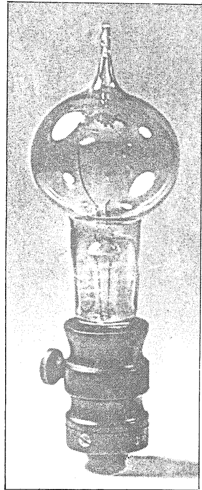
Edison's first light bulb, with carbon (charred cotton) filament and air valve in the base
