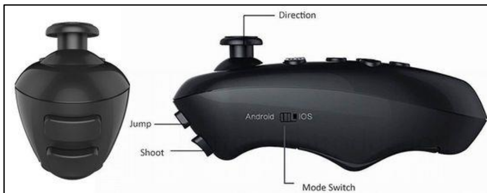
Figure 28: Bluetooth joystick attached to the 3D printed artefact (Manual) Google search: https://cdn-0.fccid.io/png.php?id=3564749&page=0
