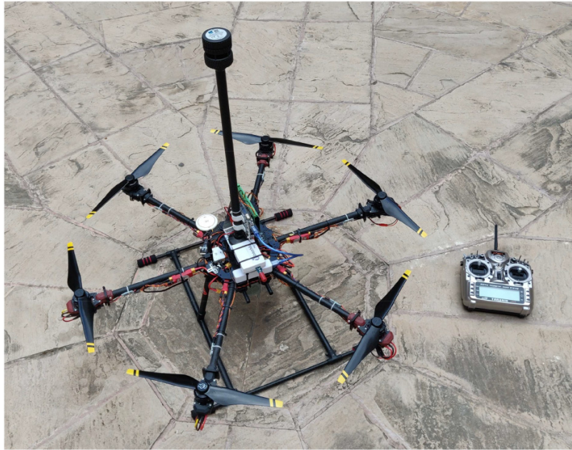
Fig. 1. The completed hexacopter RPAS setup.
