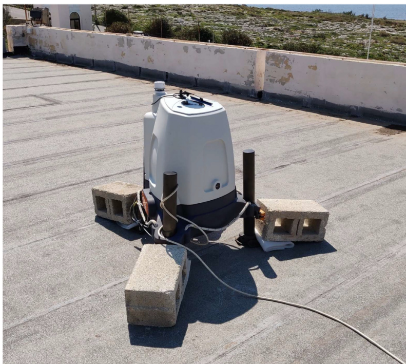
Fig. 2. The ZephIR ZX 300 LiDAR unit installed on the rooftop of a building, at Ċirkewwa, l/o Mellieħa, Malta.
