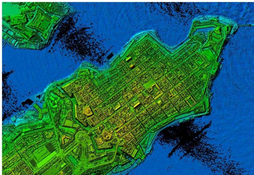
Figure 2. Lidar Data: Lidar image depicting the Valletta peninsula in Malta depicting detailed urban infrastructure, street alignment and open spaces.
