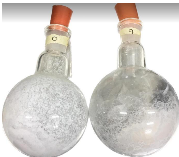
Figure 93 Figure showing white foam left behind in the round bottomed flask when freeze drying coelomic fluid from day 0 and day 9. Photo: Taken by Author.
