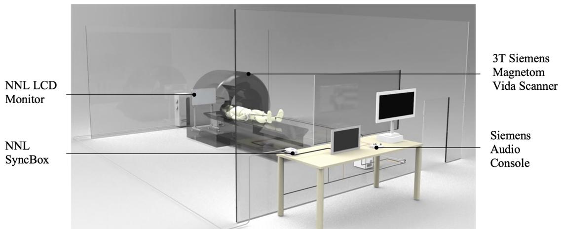
FIGURE 4.7: The MRI system layout. Adapted from [164].
