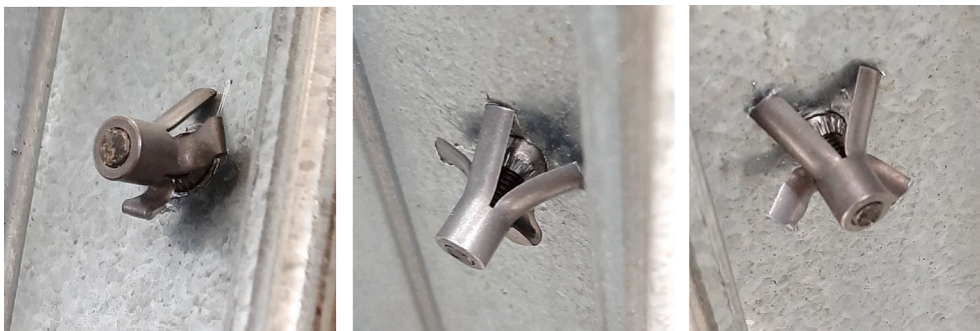
Fig. 19. Failure of specimen 2-P24-P3 showing bending of the four segments of the locking nut.
