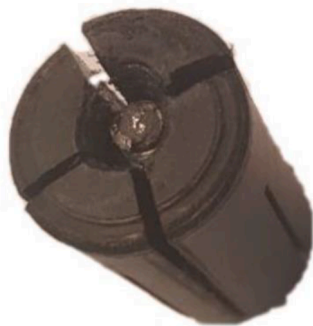
Fig. 13. Failure of specimen 1-P20-P2 – screw bearing into the preformed slots.
