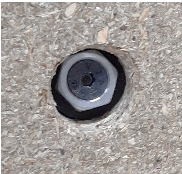
Fig. 18. Rotation and pull-through failure of specimen 2-P15-P3.
