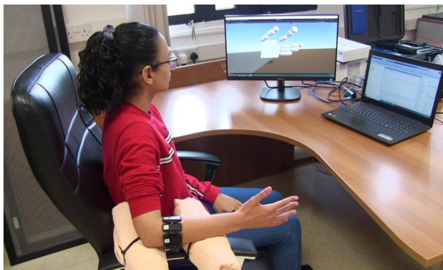
Figure 6.2 - The Testing Setup which included the seated subject with the forearm placed on the towels, with the wrist in a semi-supinated position. The Myo band was placed on the forearm bulge of the subject's dominant hand whilst not being in contact with any materials. The laptop and monitor were placed in a comfortable position for the subject to follow the experiment.
