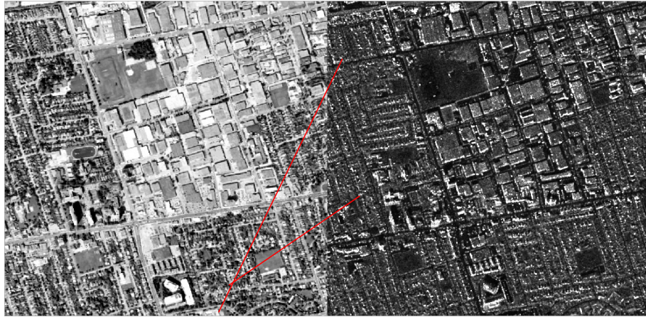
Figure 6.39: Obtained failed matches using SAR-SIFT for the RIFT dataset Optical-SAR image pair.
