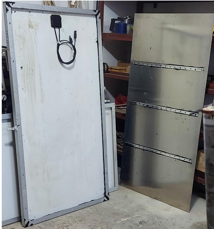
Figure 75: PV Panel with sealed internal edges (Left) and Aluminium sheet with three stiffeners attached (Right).
