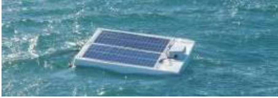
Figure 17: Offshore PV module float in Maltese seawater [10].
