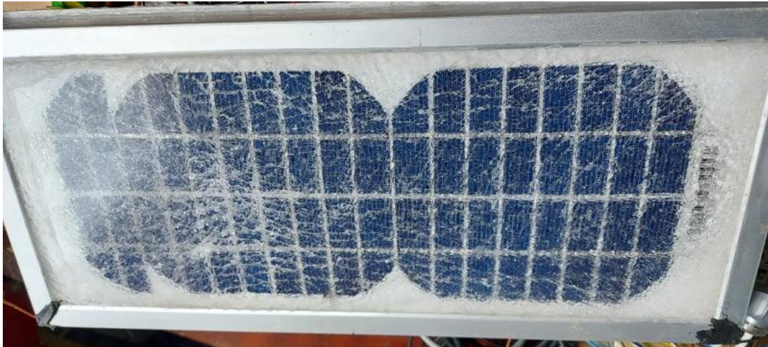
Figure 59: Shattered PV glass at 3 Bar water pressure.
