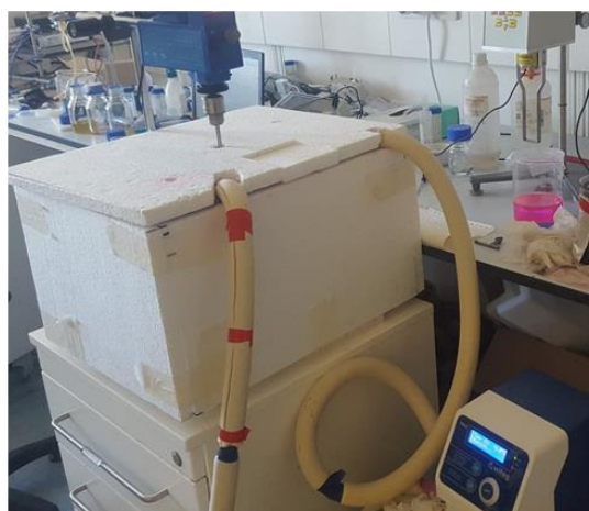
Figure III.1 (Top) Schematic of the reaction chamber (Left) Insulated reaction chamber (Right) Black solution formed at -10^{\circ}\text{C} using a 1:20 Silver nitrate: Trisodium citrate ratio
