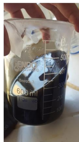
Figure III.1 (Top) Schematic of the reaction chamber (Left) Insulated reaction chamber (Right) Black solution formed at -10^{\circ}\text{C} using a 1:20 Silver nitrate: Trisodium citrate ratio
