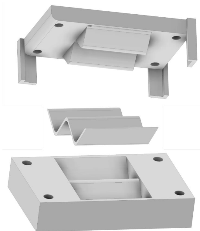
Figure 6.26.(top & bottom) CAD of the moulds used, and (middle) the ME structure produced.
