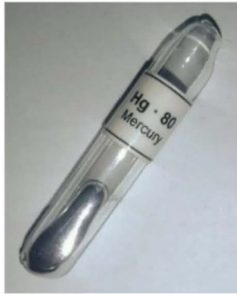
Figure 2: A glass ampoule containing pure elemental mercury. Being liquid at room temperature enables mercury to seep through any potential cracks that may form in such apparatus if mishandled, increasing the likelihood of an exposure incident.
