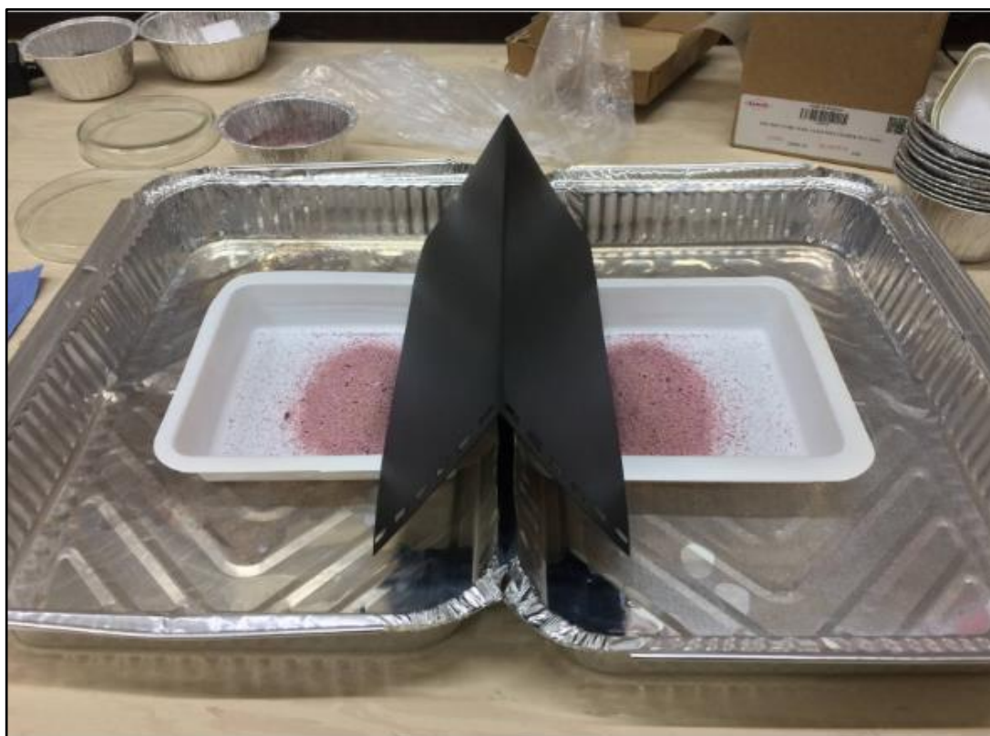
Figure 2.4.1 – Photograph showing the splitter device used for unbiased subsampling of the sediment.
