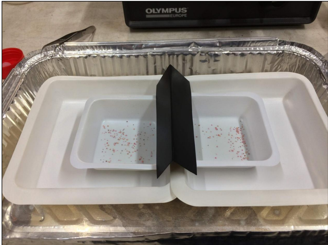
Figure 2.7.1 – Photograph showing the random subsampling device used for splitting stained Amphistegina lobifera shells for photographing.
