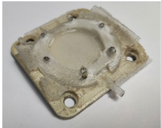
Fig. 13 Ejection side, case study 1, insert failure at first injection run
