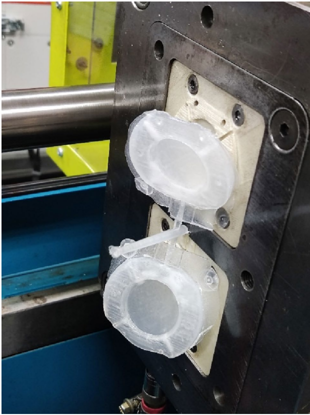
Fig. 14 Parts of case study 2 as produced during injection molding. The parts were stuck to the sides of the inserts due to flash, even after ejection
