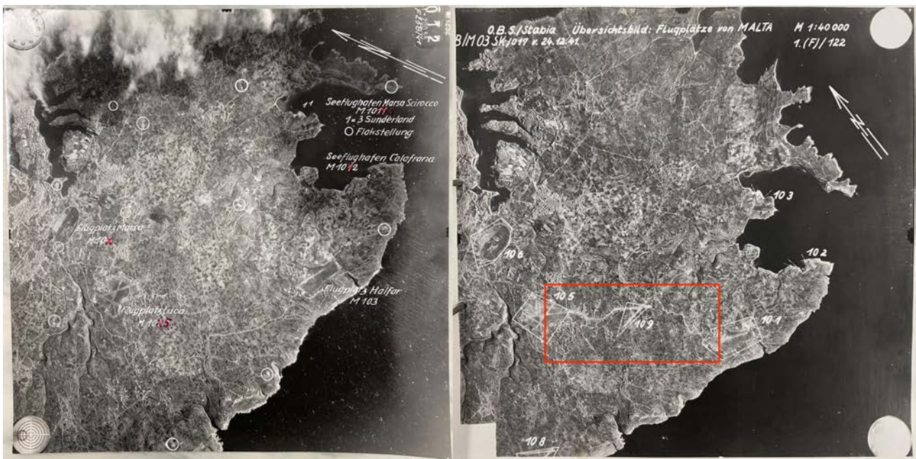
Figure 3: German reconnaissance images from January (left) and December (right) 1941 showing the creation of the Luqa/Safi/Hal Far taxiway and dispersal network (within the red box) (source: NARAA-b).
