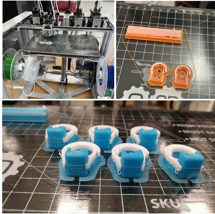
Figure 5: a) The four-head fused filament fabrication printer (b): During print (c): Post completion of print.
