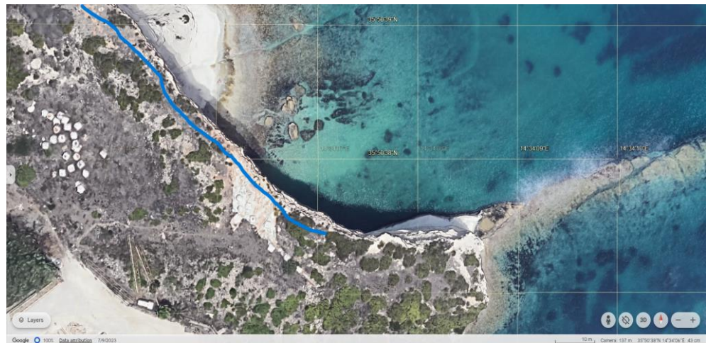
Figure 3. In this figure, taken from Google Earth, the blue line represents the major upper crack visible on site, extending to the area of the overhang with the overlying Neolithic building.
