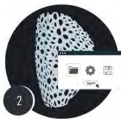
Step 2: Engineers use CT scan to create the bone scaffold's design
