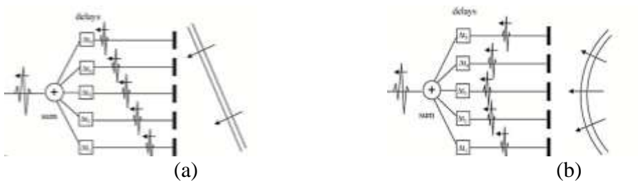
Figure K.9 ~ The phased array operations in receiving mode. It can be seen that (a) the array enhances signals received at an angle through the application of delays and summation and (b) signals being received from a shaped wave front are also similarly enhanced [155].
