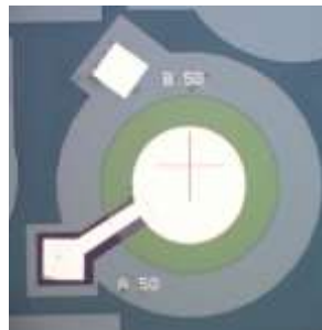
Figure 4.63 ~ Frontal device micrograph of Device 50 – 650 \mu\text{m} diameter PMUT.
