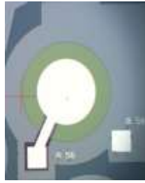
Figure 4.70 ~ Frontal device micrograph of Device 56 – 700 \mu m diameter PMUT.
