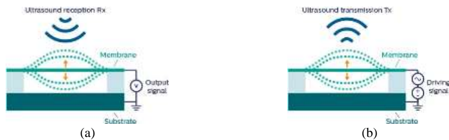
Figure 2.4 ~ Principles of operation of a CMUT showing operations in (a) ultrasonic reception and (b) ultrasonic transmission [53].
