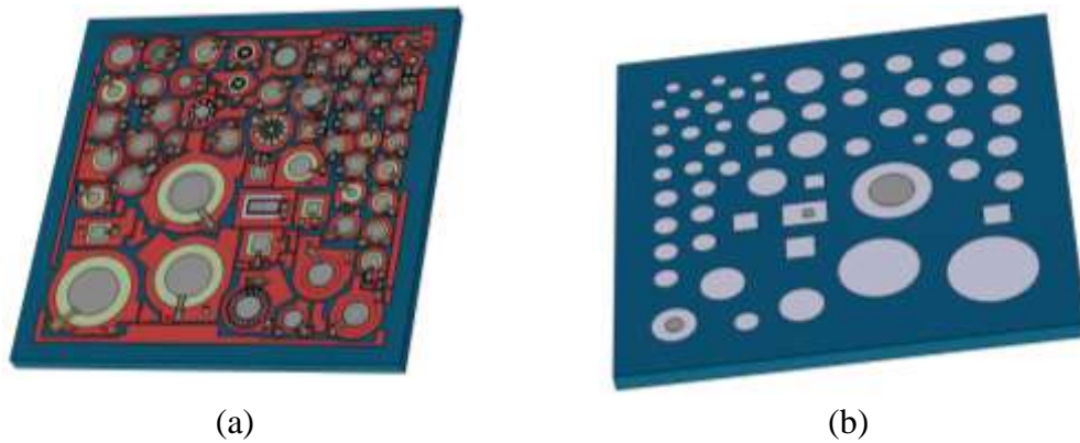
Figure 3.52 ~ A view of the digitised IC showing (a) front side (b) rear side. This model was set up for transfer into COMSOL Multi-Physics for final Finite Element Analysis to be conducted prior to production of devices.
