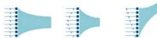
Figure K.6 ~ A schematic which shows the principles of ultrasonic beam steering and focusing in an array system [100].
