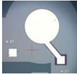
Figure 4.168 ~ Micrograph showing frontal side of device 27. Part in white shows padmetal.
