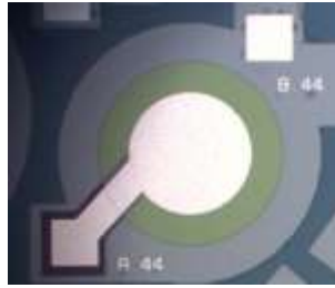
Figure 4.30 ~ Frontal device micrograph of Device 44 a 600µm diameter PMUT.
