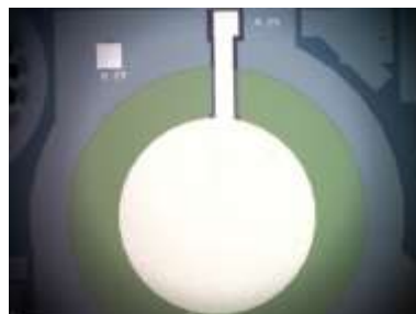
Figure 4.188 ~ Micrograph showing frontal side of Device 29. Part in white shows padmetal.
