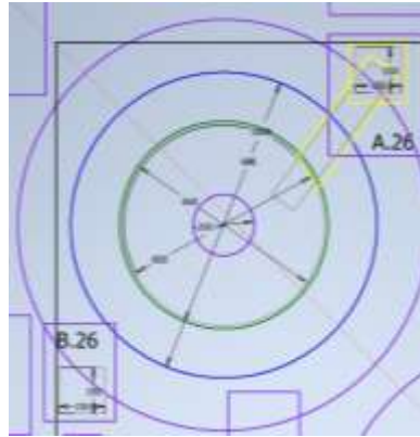
Figure 4.156 ~ Blueprint drawing of Device 26 showing the dimensions of the device including the centrally suspended mass.
