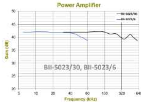
Figure 4.13 ~ The frequency response of the BII-5023 Power Amplifier [123].
