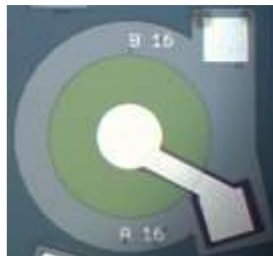
Figure 4.27 ~ Frontal device micrograph of Device 16 – 550 µm diameter PMUT.
