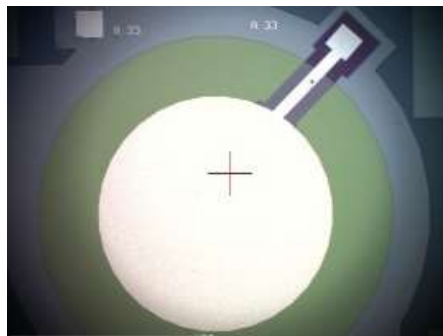
Figure 4.196 ~ Micrograph showing frontal side of Device 33. Part in white shows padmetal.
