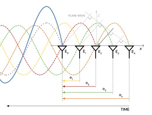
When waves from multiple sources interact, they tend to combine and interfere along many different directions. The process of constructive interference is when the peaks and troughs of individual waves add up to create a stronger resultant wave in a particular direction. Using the phased array, we can control that direction by adjusting the relative phase of each individual source in the array.
