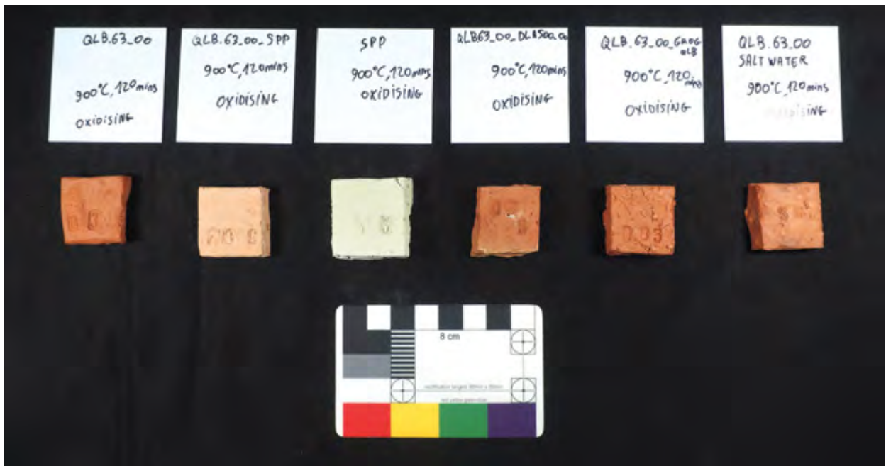
Top: Experimental briquettes made with different possible raw materials from Malta. Photo by Kellian Coste (Intern - University of Edinburgh)
