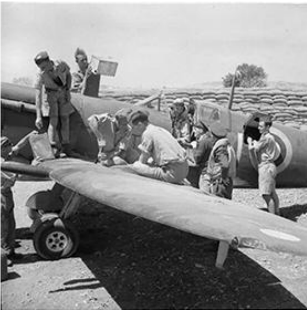
Ground crew rearm a Supermarine Spitfire Mark VC of No. 601 Squadron and refuel it using four-gallon petrol tins. Flight Lieutenant Dennis Barnham is in the cockpit. Photo: ww2today.com
