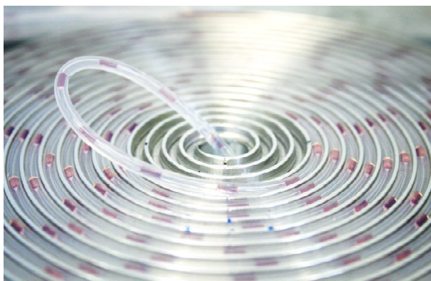
Figure 1. Continuous-flow spiral-shaped microphotoreactor for gas-liquid photooxygenations (LGC, Toulouse).
