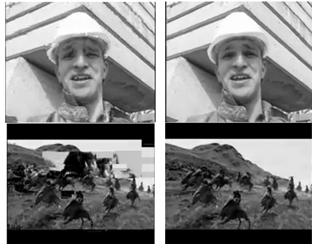
Fig. 8. Video sequences from (a) Foreman and (b) Lord of the Rings (Two Towers) using (left) Standard decoder and (right) HECAD algorithm.
