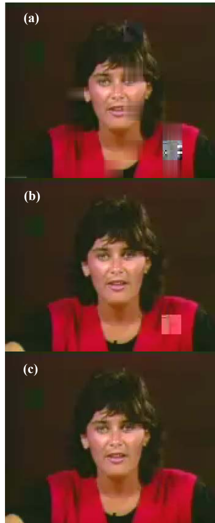
Fig. 6. Frame 5 for the Miss-America sequence (a) MB Level concealment, (b) proposed List Decoder, and (c) proposed decoder with AIDB detection
