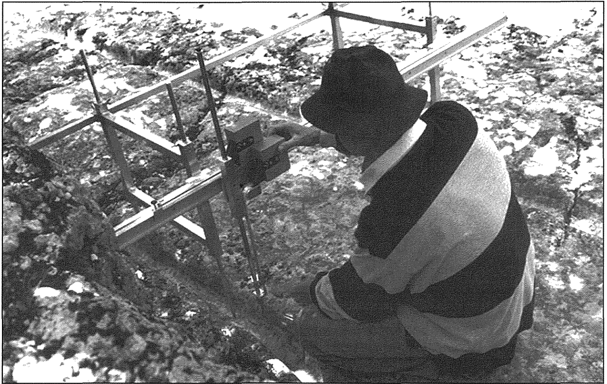
Plate 1: Instrument for measuring cart-rut profiles
