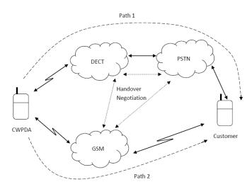
Fig. 1. A combined DECT-GSM wireless access system.
