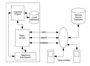
Fig. 3. The proposed ACMR architecture and its connection to networked components and other ACMRs.
