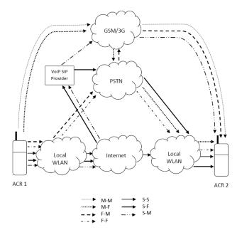
Fig. 2. The ACMR in a system that comprises cellular networks (M), PSTN switched systems, internet systems (S) and low-power radio systems that piggyback on fixed PSTN lines(F).
