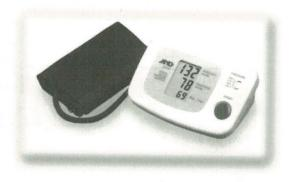
The UA-767 has one button operation: Power-on, start, pressurisation at preset level, automatic measurement, display of systolic and diastolic blood pressure readings and heart rate, automatic cuff deflation and unit shut off are accomplished with the push of only one button.
