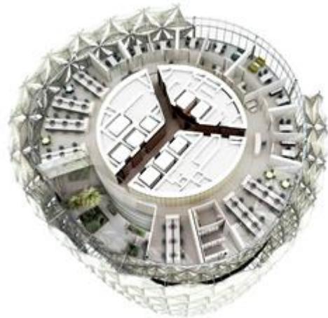
Figure 5: Axonometric view of tower showing typical office floor layout at skygarden level
