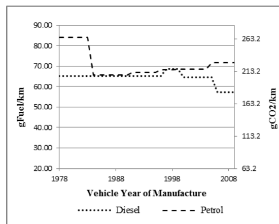
Figure 4 Modeled Average Consumption & Emission Factors for Passenger Cars by Year of Manufacture in Malta (based on EMEP/EEA emission inventory guidebook 2009.)
