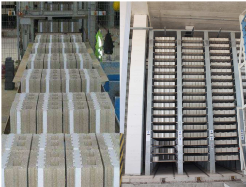
Figure 7, 8: Dry mix compaction & casting of Thermablocks, 4 in a row, stacked for curing.
