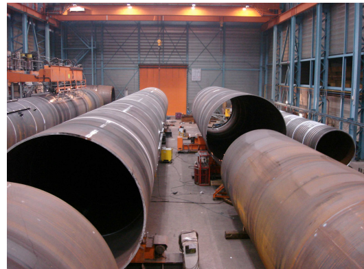
Figure 6: The individual cans are aligned and welded to form the monopiles
