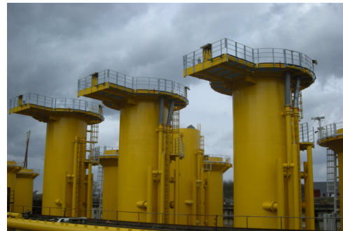
Figure 2: Transition pieces awaiting transport
