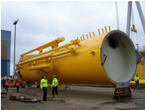
Figure 7: Transition piece at the fabrication yard ready for upending
